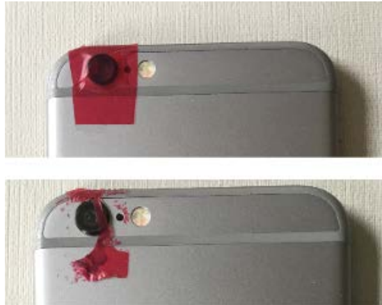
Figure 3: Sealed smartphone camera (intact and broken)
